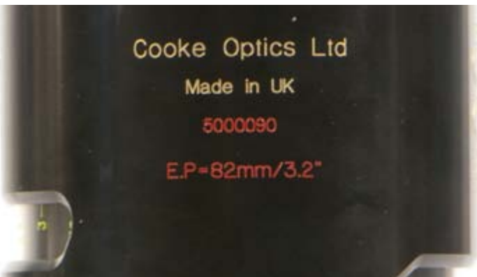
Below: Helpful notation of Entrance Pupil (E.P.) position in mm and inches from the lens mount flange. This is the optical "pivot point" to be centered on nodal heads to eliminate image shift when panning.
