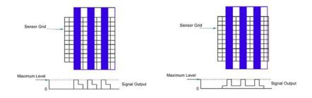
The distorted signal results in jagged edges very noticeable when the lines are at a slight angle with the sensor grid (effect that is called aliasing) and the reduced amplitude is a reduction in contrast that negatively affects the resolution perception.
