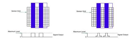
The signal can still have a significant amount of distortion (aliasing) but the white is at full level and the black reaches the 0 level.
