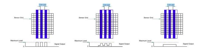
But as it gradually shifts from alignment, the signal deteriorates to the point of not showing any detail. This is an illustration of the Nyquist theorem that in essence states that at a given frequency a signal (in this case a repeating pattern of line pairs) needs <u>more than two samples per cycle to be properly represented.</u>
