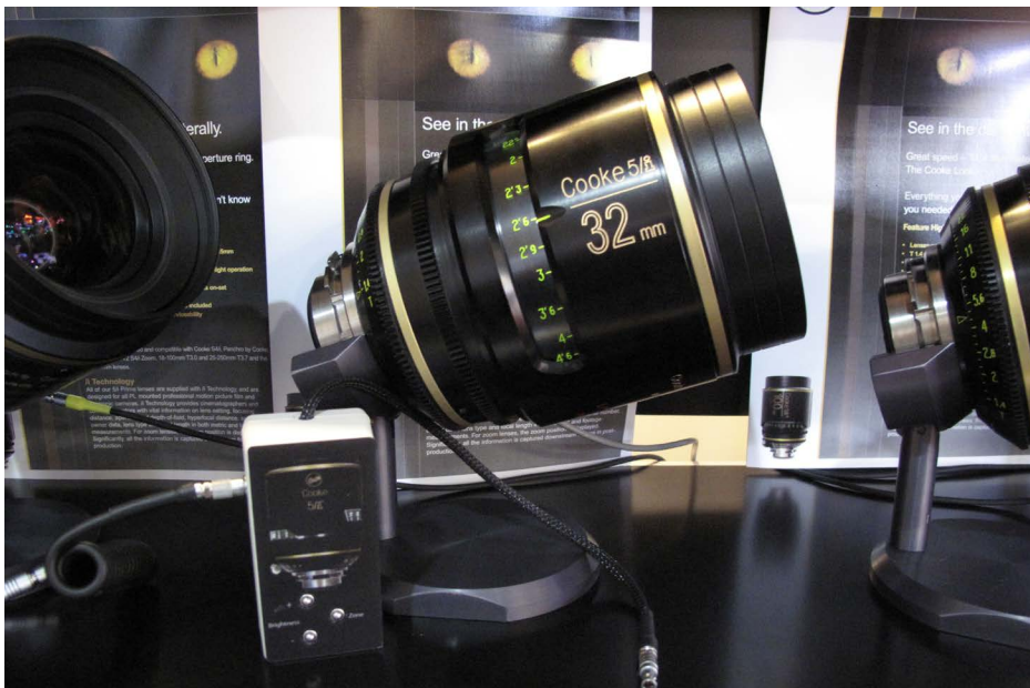
Small external /i lens dimmer box for Cooke 5/i. Also on display were controls to dim and display data from Preston Cinema Systems, cmotion and Transvideo.
