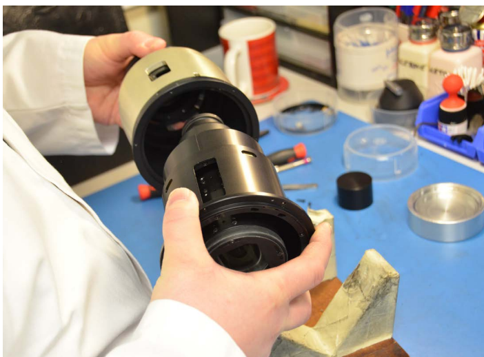
The "Inner" being mounted into the "Outer"
