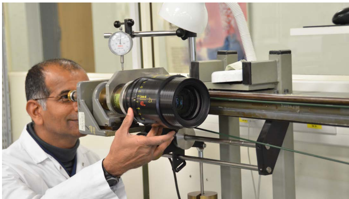
1. In the lens assembly area, Raj Mistry calibrates the focus scale individually for each lens.
