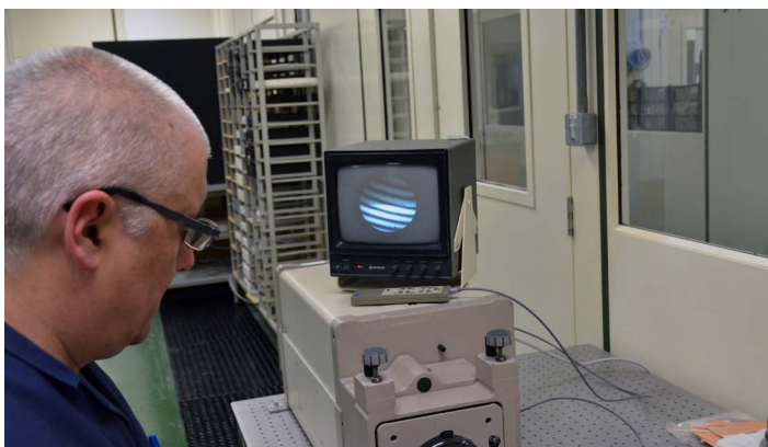
Chris Norton inspects the form of a glass element on a Zygo interferometer
