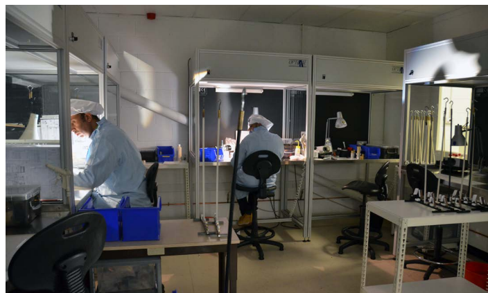
Glassing up the inner is done in a clean room
