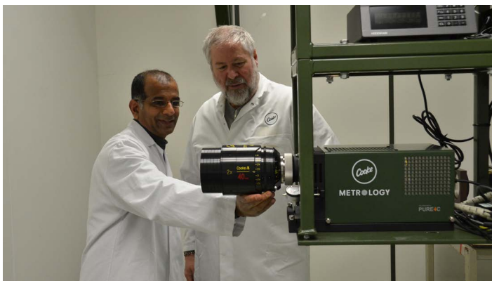
5. The lens is mounted and the focus scale set to 3 feet.
