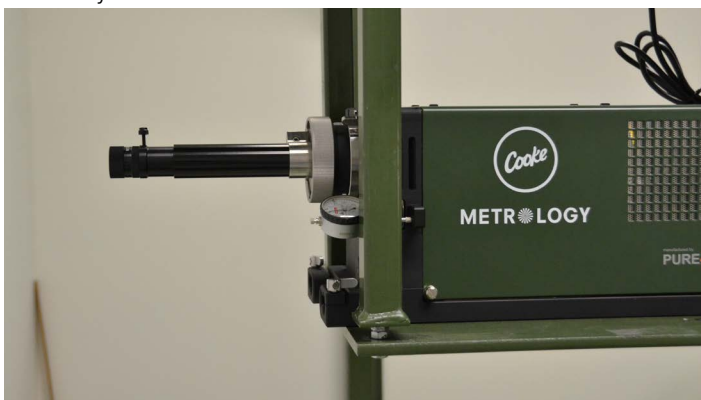
3. On the projector, made by Cooke Metrology, of course, the flange focal depth is checked to be sure it is exactly 52mm.
