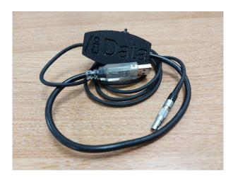
The button in the middle of the new cable is useful for interrupting power to the lens when running the Cooke /£ Update program to update lens firmware.
