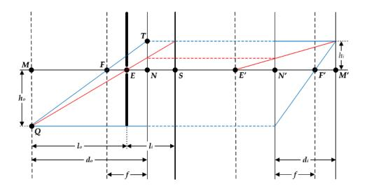
We now have enough information to define the pinhole focal length  $l_i$  in terms of the thick lens model. Start by noting that QMF and TNF are similar triangles. This means that:
